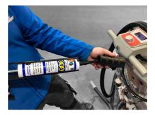
Cut suction hose to desired length and fit universal fitting so this can easily be fitted into the suction tank. We recommend CT1 adhesive for glueing the hose connector to hose).
