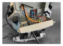
Find the cable and water pipe entry point into the battery compartment. Rear casing or handle assemblies often have entry points you can also drill through switch plates, as shown, for access.
