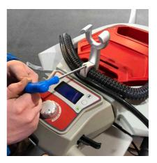
Clamp the hose in to place on the upper machine mount.
