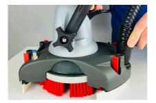
Attach the brush; Hold the hub stable with one hand and twist brush until it locks
