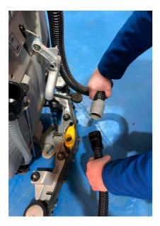
interval to fit various tanks. If the suction tank inlet is not easily accessible you can fit the Force hose onto the squeegee hose as shown.
