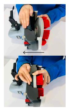
4. Lift machine out of lower mount
