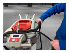
Separate the suction hose and cable/ water pipe hose.
