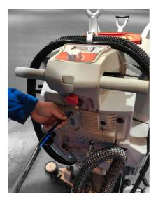
Insert the cable/water pipe into the machine so it goes into the battery compartment.
