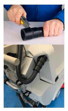
The majority of machines have a suction tank inlet conveniently at the back, high up near the controls. MotorScrubber Force universal adaptor will fit the majority of machines with female or male connections. You can cut down the fitting at each
