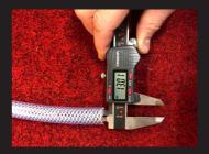
Measure the internal diameter of the water pipe which exits the water tank.
